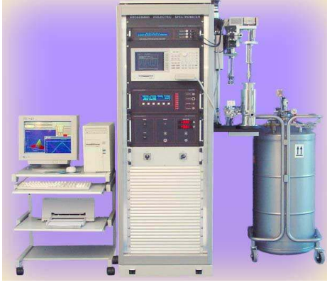
Figure 1. Novocontrol Alpha Dielectric Analyser
